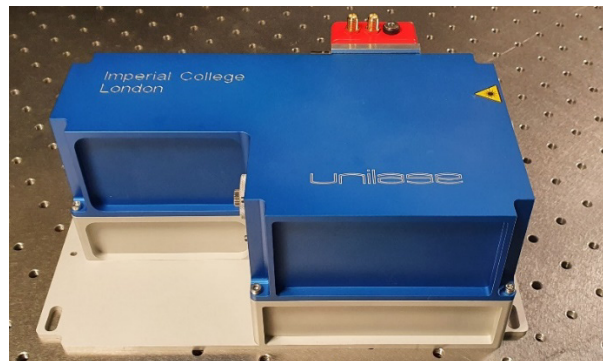
Figure 5: Photograph of fully packaged diode-pumped Alexandrite laser.
